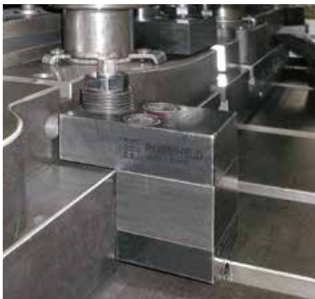
Use of mechanical sliding clamps on a machine table
