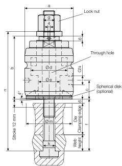
Freely adjustable and flexible adaptation to suit varying heights of clamping edges of the dies by quick and easy adjustment of the tie rod by means of a lock nut.
