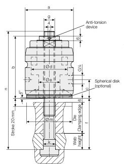
Optimum adaptation to varying heights of the clamping edges of dies by an increased total stroke of 20 mm (higher total stroke on request).
