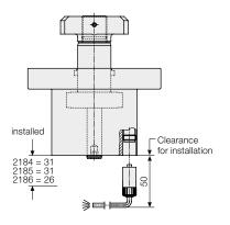
Both proximity switches are connected to the base of the pull clamp through a connecting cable with screw coupling [IP 67].
