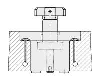
Hydraulic oil is fed through the drilled holes in the bed and in the ram. There are no exposed pipes or fittings. The sealing is made by O-rings supplied with the clamp.
