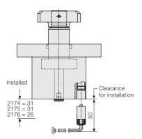
Both proximity switches are connected to the base of the swing clamp through a connecting cable with screw coupling [IP 67]. Please order the connecting cable separately. Further installation may be carried out using a distribution board with an LED display.
