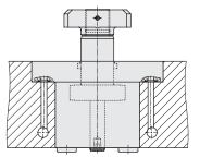
Hydraulic oil is fed through the drilled holes in the bed and in the ram. There are no exposed pipes or fittings. The sealing is made by O-rings supplied with the clamp. Easy installation, ease of servicing.
