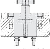
Pipes are recommended in applications where fittings are easily accessible and where pipes do not impede installation and dismantling of the swing clamps.
